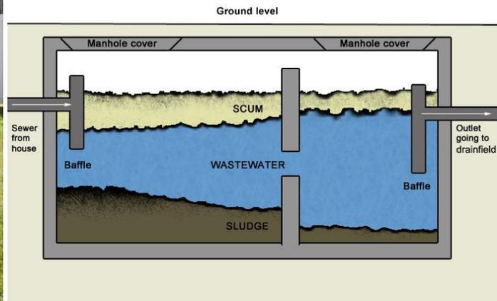
Septic contractors were met at properties where the septic tanks needed pumping. The layer (scum, liquid, sludge) thickness was measured for each tank and samples of the layers were collected for nutrient analyses. The volume and concentrations were used to determine masses of nutrients pumped from the tanks.
